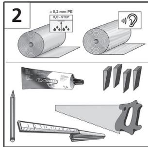
**Preparation:** Please store the packets 48 hours prior to installation under the same climatic conditions (temperature and moisture) as the actual installation process [1]. Important pre-condition for proper fitting and long-term durability of the laminated flooring is a room temperature of ca. 20°C/68°F and a relative humidity of around 50 – 70%.
